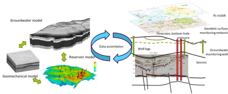
Figure 1: Integrated approach for subsidence estimation.
